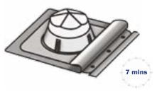
Roll down and seal the skirt against the roof membrane and roll in seal.
