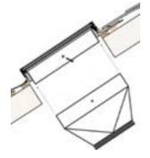
Using the clear mastic from above, seal the gap between the transition and the wooden frame.
