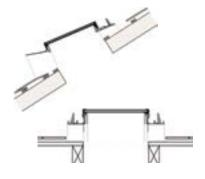
With the rooflight face down to the floor, unfold the lead flashing along the lower edge so that it is flat. Located on each of the two long sides of the rooflight are two metal brackets. Fold each of these up so that they are at a 90° angle to the flashing plate.
